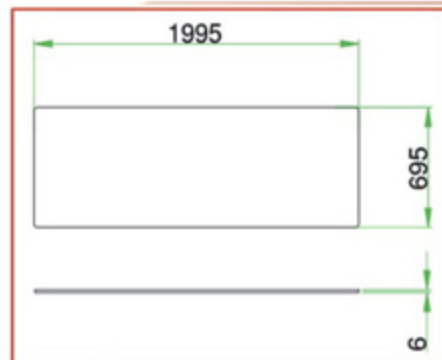
MF-PG2000-01 Copertura in gomma stampata anti-olio per banco MF-BL 2000 Dimensioni 1995x695x6mm Oil resistant moulded rubber cover for MF-BL 2000 workbench. Dimensions 1995x695x6mm
